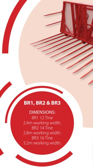
Moulton push off Buck Rakes are of heavy duty construction, using twin double acting rams and are fitted with 1.4m conus 2 tines fitted into tapered bushes.
