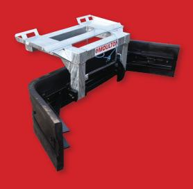
SP1 feed/silage pusher designed for pushing back'nosed' out feed closer to the feed barrier. The SP1 incorporates twin wheels fitted with used super single lorry tyres.
