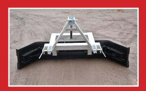
The YS4-HGP Yard Scraper is fitted with a 50mm, moulded rubber blade. The blade is designed to turnover allowing use in both forward and reverse, a travel direction lock is realised by a rope from the tractor seat.
