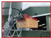
The BBG2 is designed to handle 3 smaller high density bales up to 900mm wide, or 2 larger 1200mm bales. Bales may be handled in both directions relative to the back frame. Our BBG range of grabs incorporate our specially designed HARDOX steel claws.
